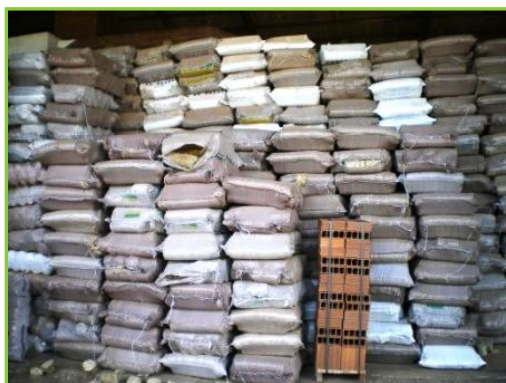
Packaged sugar cane bagasse “brickets” at the facility, waiting to be used as fuel in the kilns
